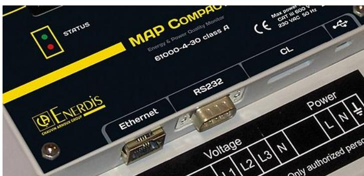
Figure 8 - Les ports de communication
