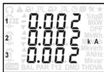
Here, the chosen caliber will not permit accurate readings of the current measured,
