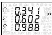
Here, the Power Factors of phases 1 and 2 are abnormally low, which may be due to inversion of the sensors on these two phases.
