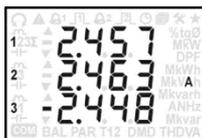
Here, the current on phase 3 is negative, which means that the flexible current sensor on this phase may be installed the wrong way round or incorrectly connected.
